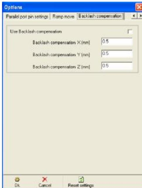
Select use backlash compensation to remove backlash out of the axis. Make sure if this option is selected that the backlash is correct, otherwise each move will contain an error.
