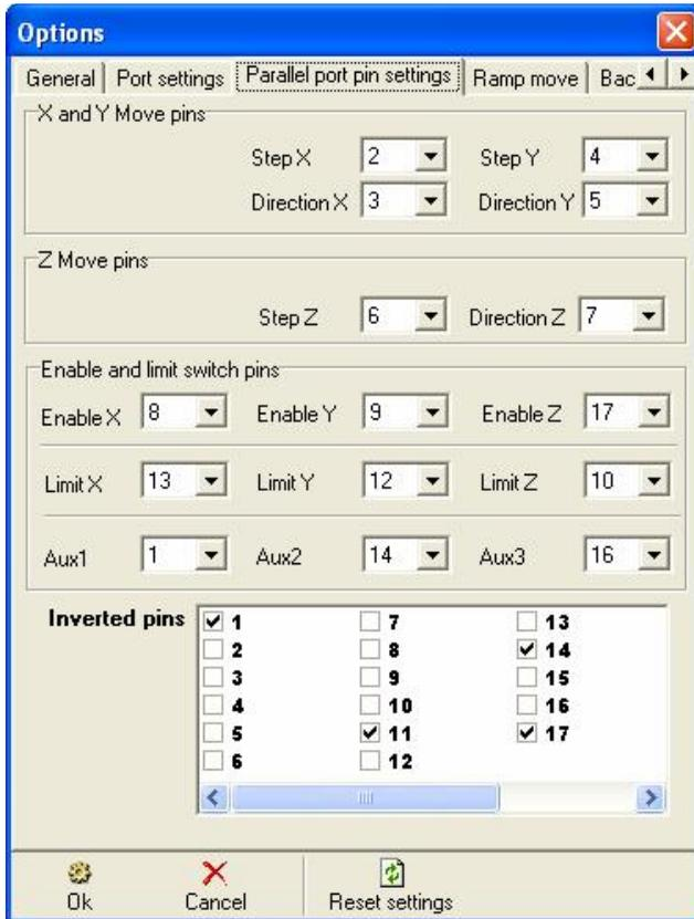
Port setting page is used to set up the various output / input pins on the parallel port for the step, direction, limit switches etc. Please note these should not need to be changed unless you are configuring it to an existing system and that differs from the default shown. You also get the option to invert pins so that there function becomes inverted.
