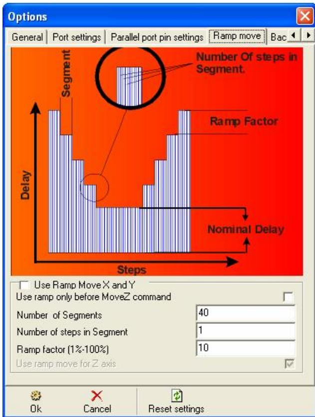
From this screen you can select to enable / disable Ramp move. Enabling this will start the stepper motors slowly then ramp up to the maximum speed (MaxSpeedTravelXY / MaxSpeedCuttingXY ) and at the end of the cut / movement the motors will ramp down the speed. Do not have move ramp only before MoveZ command enabled/
